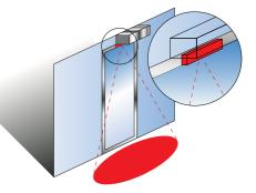
Optic sensors with selectable function "Reverse" or "Stop" provide additional safety in the event of pinch points or oncoming traffic.
