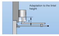
The progressively adjustable standard rod assembly (measure X) and the axle extensions (measure Y) provide the suitable solution for each construction situation.
