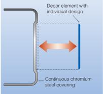
The decor element is glued onto the chromium steel covering.
