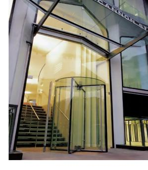
The Crystal TQ uses a combination of tempered and laminated safety glass. The doorset is made from 1/2" tempered glass connected to the center stainless steel shaft with specially made stainless steel clamps. The 11/16" tempered laminated glass ceiling is fixed directly to the curved laminated glass sidewalls with small, unobtrusive clamps. Tinted glass is available.
